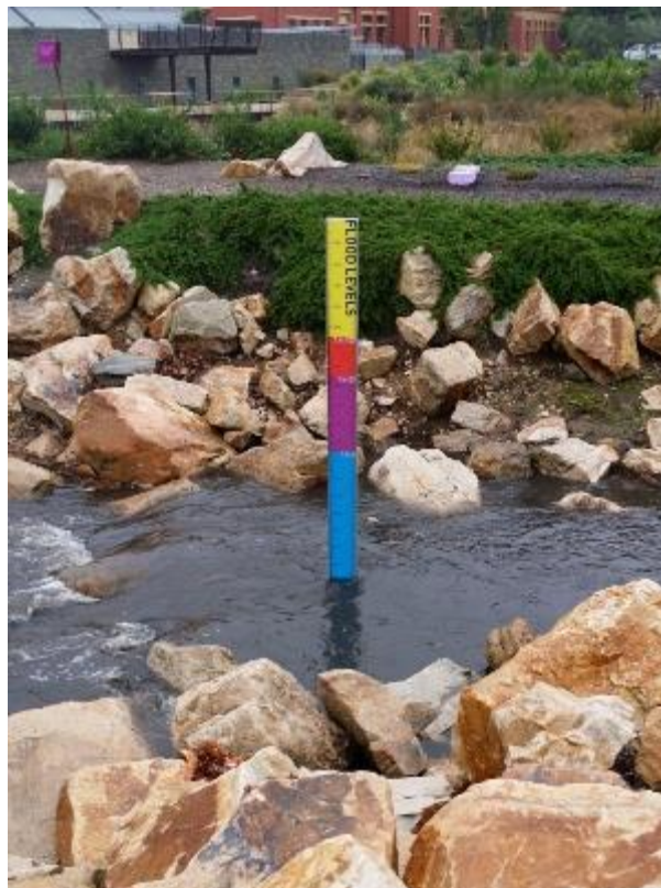
Figure 81: Flood level indicator, with red highlighting the 1 in 100 year flood event level. (Hydro-Future 2015)
