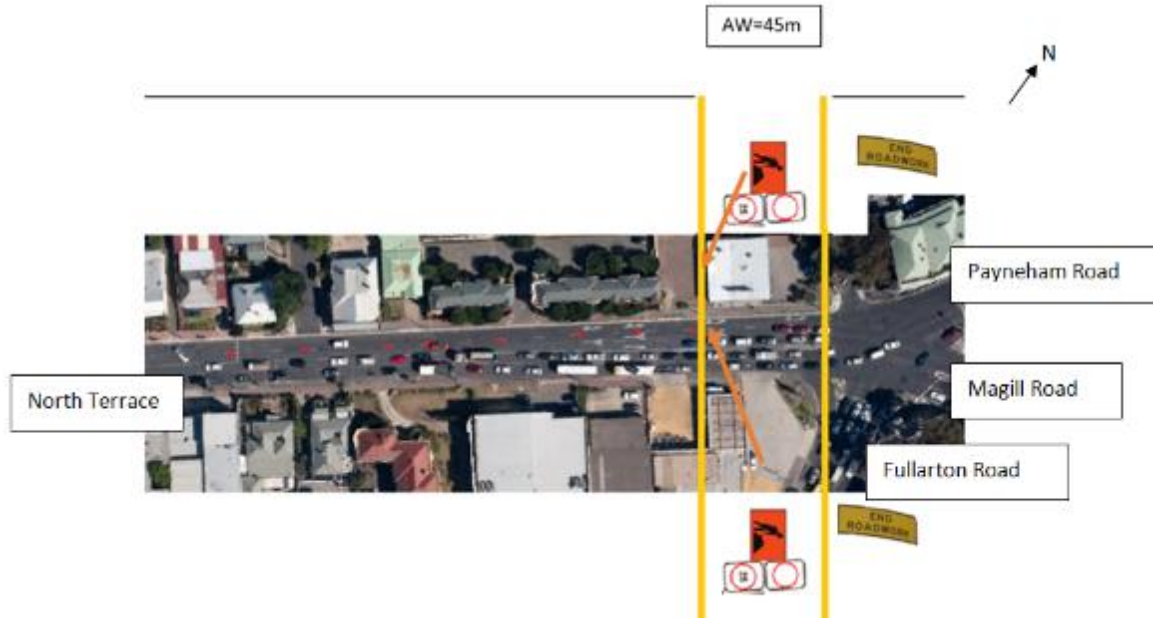
Figure 182 Workzone Setup-One Lane Closed Outbound -End of Works
