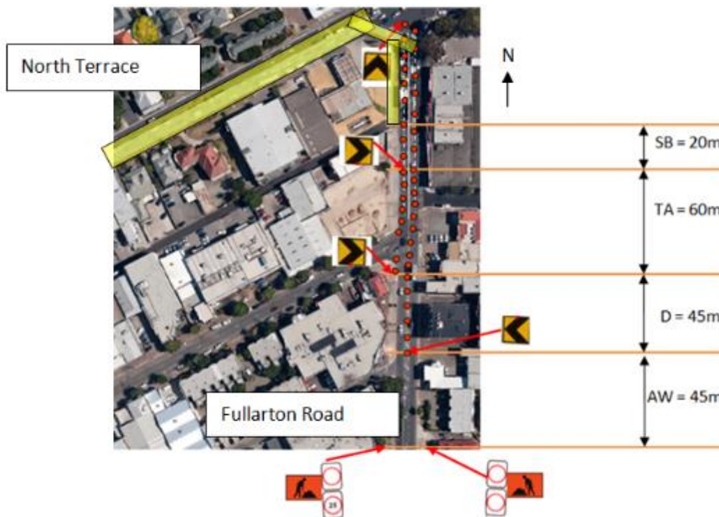
Figure 190 Workzone Setup-Two Lanes Closed Inbound-Fullarton Road Approach
