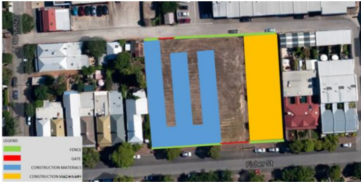
Figure 225 Location of the site yard (Google Maps, 2015)
