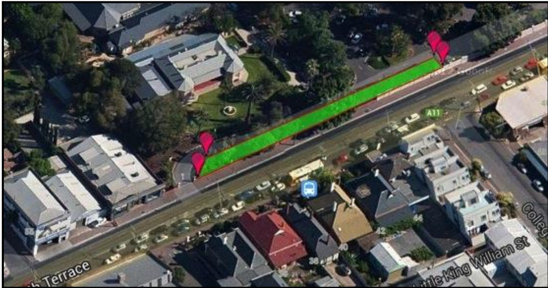
Figure 66: Area that could be used for bio-retention basin (in front of St Peter's College)
